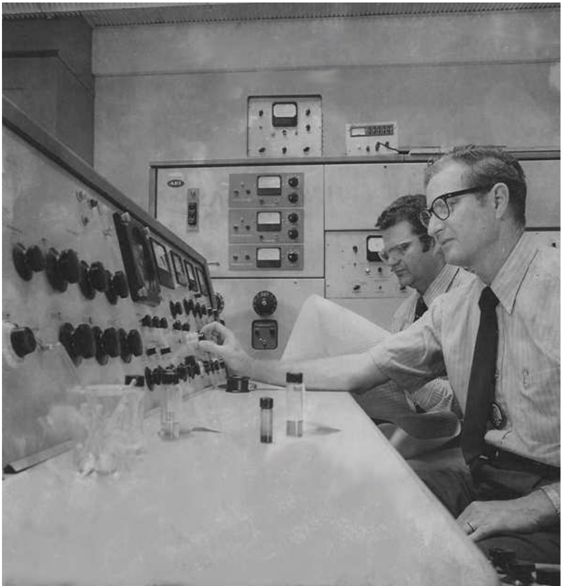
Lumpkin and Thomas Aczel using an Associated Electrical Industries [AEI] MS-9 mass spectrometer, June 1974
