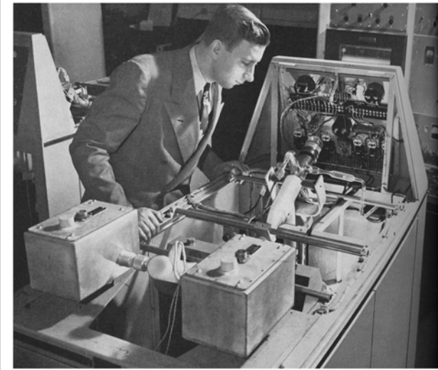
FOR ANALYZING GASES BY SPECTROMETRY Measurements of impurities in gas streams, certain analytical work in the rubber and petroleum industries, and other types of gas analysis are among the many applications of recording mass spectrometers of the latest type, one of which is shown here being inspected in the laboratory.
