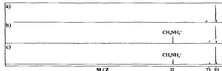
Figure 2. EI mass spectra of aniline with reagent gases. a) ammonia Proton transfer is not observed b) methylamine using pulse sequence I. Protonated methylamine \text{CH}_3\text{NH}_3^+ is observed, suggesting that the proton affinities of the radical cations, or protonated form, or the fragments of aniline lie between ammonia and methylamine. c) methylamine using pulse sequence II. Protonated methylamine does not increase, confirming the proton affinity of the radical cation of aniline is higher than aniline
