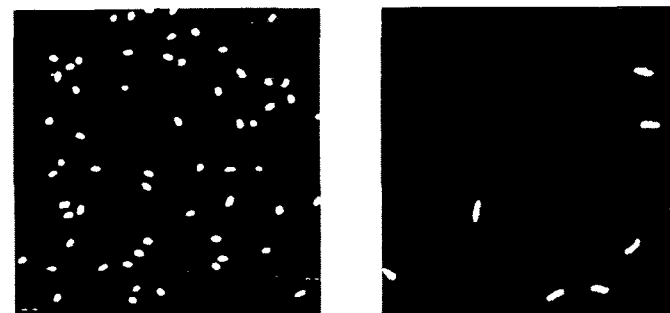
Fig. 1 TM-SFM images (500 nm by 500 nm) of hillocks generated on HOPG by impacts of 146 keV disulfide-intact charge state +9 (right) and disulfide-reduced charge state +14 (left) lysozyme.
