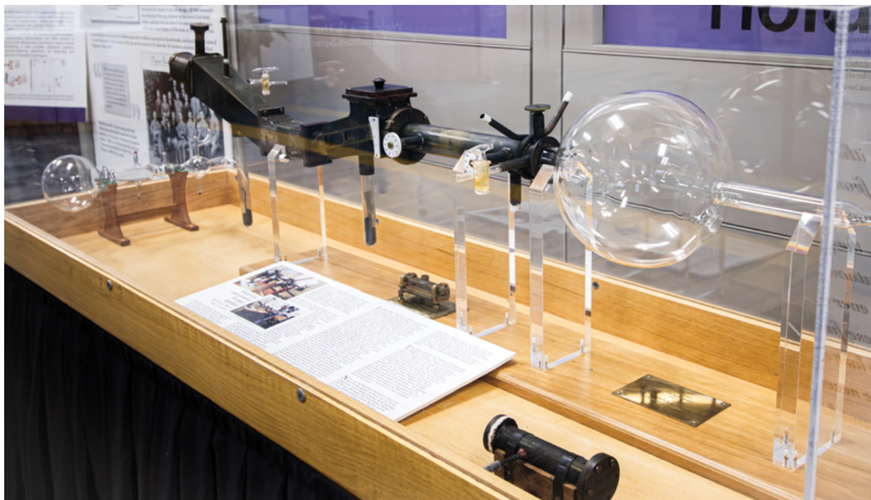
Replicas of three important historical instruments: the cathode ray device used to discover the electron (left), the Aston's mass spectograph (long instrument, center) and Chadwick's neutron chamber (foreground, right) are currently on display at the J.R. Oppenheimer Center.
