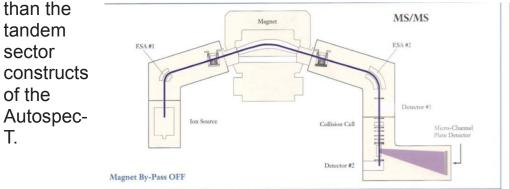
Ion optical arrangement of the Autospec oa-ToF
