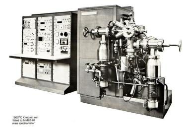
Subsequent VG 70-70 with Knudsen cell iterations of the 70-70 were engineered in the horizontal plane, and changes were made in the vacuum pumping to accommodate chemical ionisation. The first of these was delivered to the Department of Pharmacology at Oxford University in 1975, and presented to the Museum of Science and Industry in Manchester, England when it was decommissioned in 1995.
