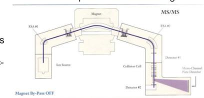
Ion optical arrangement of the Autospec oa-ToF
