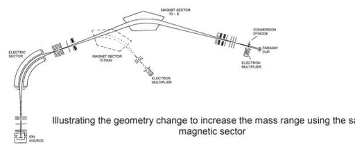
The same principle of rotating the magnet pole faces to extend the mass range was also applied to the ZAB series of instruments, with the ZAB-SE including a 26" radius high-field magnet delivering a m/z range of 15,000 at 8kV accelerating potential.
