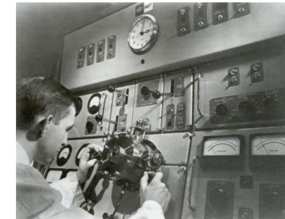
MS7: The spark source Mattauch-Herzog type double focusing sector instrument operated by J. Rogers Woolston at RCA, USA, for analysis of solids in 1961. The first MS7 to reach North American shores, it shared its DC7-F (freighter) plane flight across the Atlantic with cages containing 100 screaming monkeys. In later years, Woolston delighted in telling the story of going to Idlewild (now JFK) airport to rescue 'his baby.'
