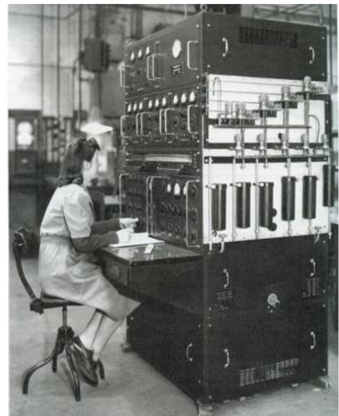
MS1 (1946): Analysis of isotope ratios in uranium hexafluoride (UF 6 ) contained in gas cylinders on the side of the instrument by mathematician Anne Mettrick from MV. This is likely to be the fourth MS1 which remained at MV and was used to develop MS2
