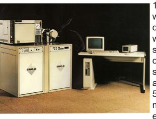
984 was the TRIO 3 with dual optical detectors and controlled with a PDP11/73 data system. The dual detectors permitted switching between MS and MS/MS modes in 50ms, and allowed mixed mode scanning experiments as well as
