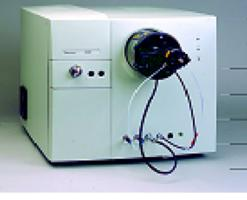
ZMD 2000 accurate mass measurement (<5ppm to m/z 500) in a routine environment using 18-bit Digital to Analog converters(2).
