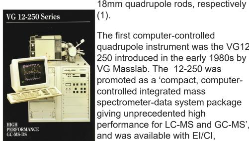
he first computer-controlled uadrupole instrument was the VG12-250 introduced in the early 1980s by /G Masslab. The 12-250 was promoted as a 'compact, computercontrolled integrated mass spectrometer-data system package
