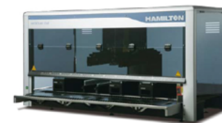
Robotic Liquid / Magnetic bead handling in 96w plates
