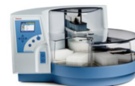
Robotic Liquid / Magnetic bead handling in 96w plates
